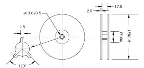
Dimensions are in mm. Tape is compliant to EIA-481-A.
