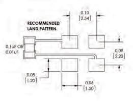
An external bypass capacitor  $0.01 \mu F$  is required between Vdd and GND
