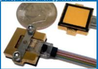
4 channel (each 12 Gbps) Transceiver for Rapid IO, PCI, Ethernet Applications
